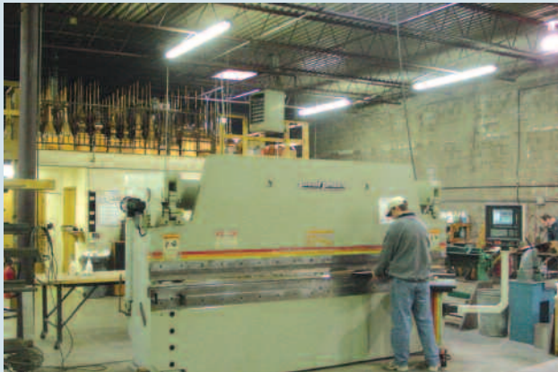
CNC Accupress Press Brake — up to 12' capabilities
